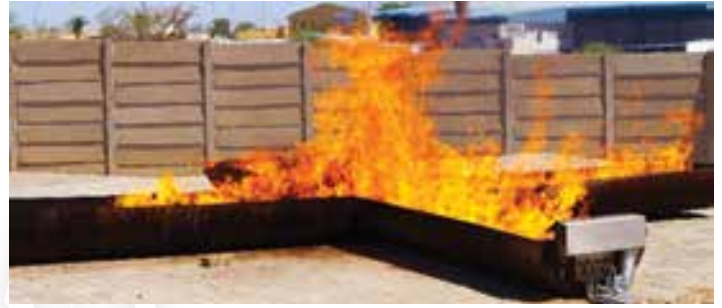
Figure 1 & 2: simulation of the devil cross, where firefighters practice on how to extinguish liquid substance fires.
