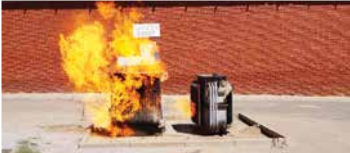
Figure 3 & 4: simulation of an electric transformer box fire; which has both the dangers of alive high volatage and flammable fluids.
