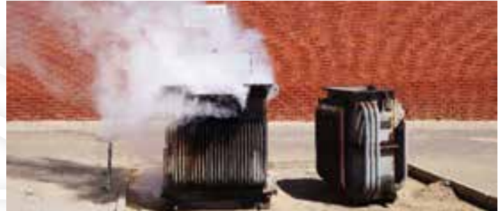
Figure 3 & 4: simulation of an electric transformer box fire; which has both the dangers of alive high volatage and flammable fluids.
