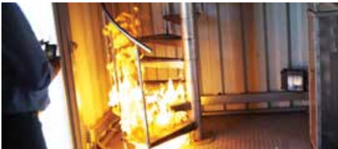
Figure 5,6,7 & 8: Simulator House, with the different fire behaviors, of rollover, backdraft, staircase fire and LPG bottle fires.
